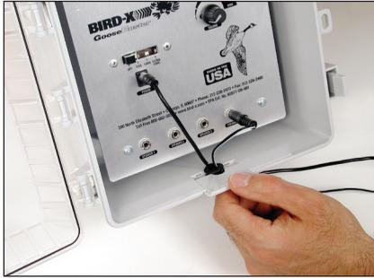
Open the control unit by lifting (releasing) the two latches on the side of the enclosure. Be certain that the power switch is OFF. Plug the four speaker wires and the AC power adapter (or DC timer with battery cables) into their respective jacks on the control panel, then route all wires down through the bottom hole cutout of the enclosure. Latch the cover.
